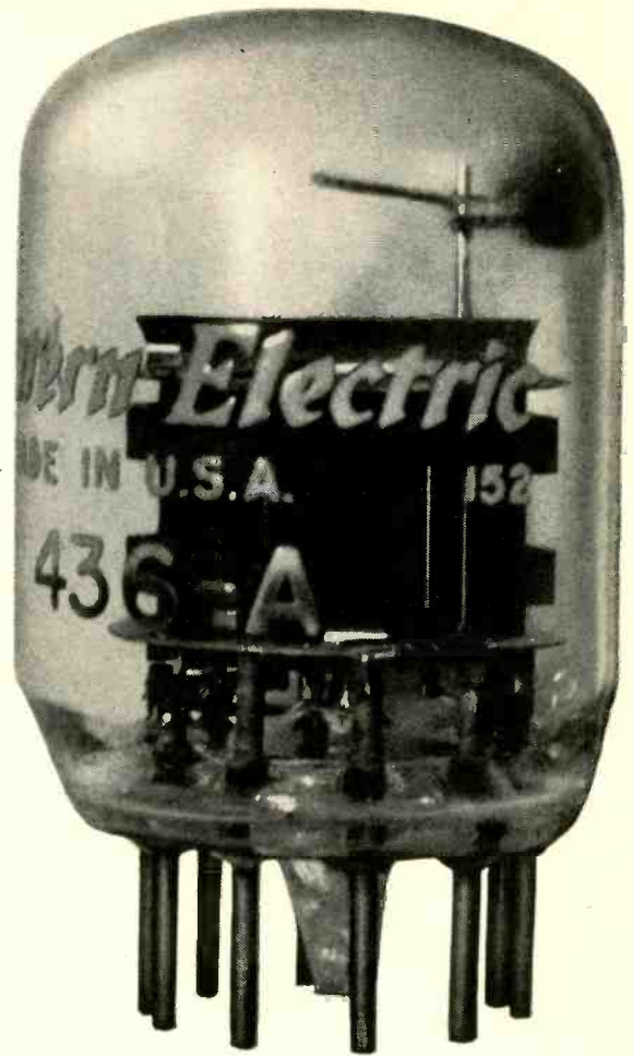
This coaxial system electron tube amplifies more voices at the same time because of wider frequency band—made possible by bringing grid and cathode closer together.
