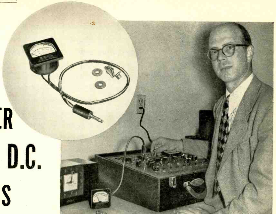
Using ammeter and checker to measure filament current. Components for modification are shown.
