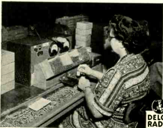
FINAL TEST ON IRON CORE ASSEMBLIES AT DELCO RADIO. Here, all iron core assemblies are carefully checked for permeability and separated into very narrow tolerance permeability groups.
